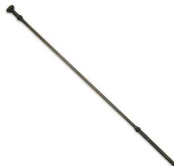
TIRANT POT DE SUSPENSION ARRIÈRE 2CV ET MÉHARI 635 MM
